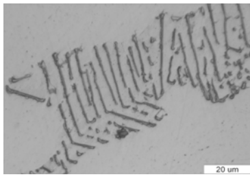
Fig. 6. Microstructure of cast steel 4.4: temperature of solutioning 950°C, temperature of ageing 450°C, 500x
