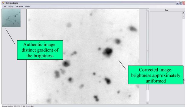
Fig.3 Model result of lighting unevenness correction.
