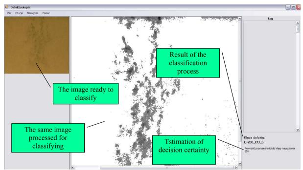
Fig 7. Result of the classifying process
