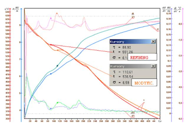
Fig. 1. Crystallization curves for the alloy AK64 cast into the ceramic moulds
