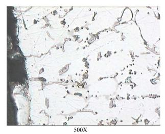
Fig. 4. Shapes and distribution of the retained impurities in the ceramic filter cast with the alloy studied
