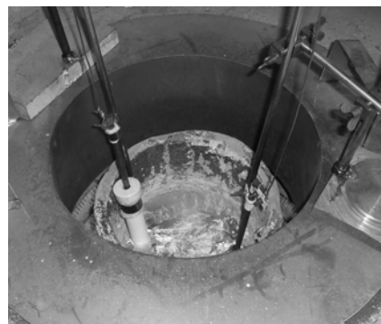
Fig. 2. View of the test stand – retort and electrode (cathode) immersed in liquid alloy
