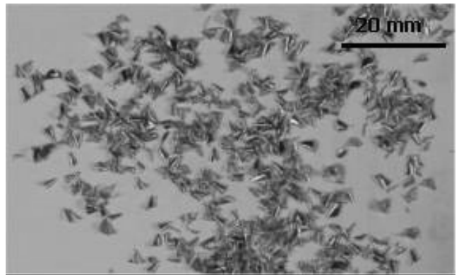
Fig. 17. Chip shape for classic leaded brass CuZn39Pb2 alloy
