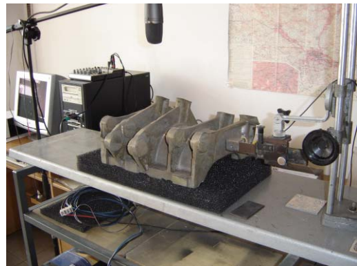
Fig.4. The technique of fixing a 2-rib casting. The selected spot where vibrations are induced in the casting.
