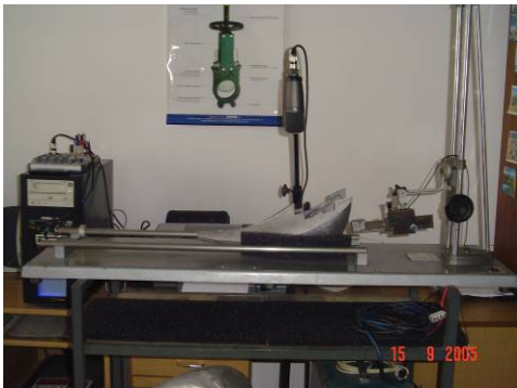
Fig. 2. A view of the measuring instruments used during sonic testing. Note a directional microphone for picking up of the acoustic field, a measuring rig with casting (aluminium alloy) placed in position, and a device for mechanical excitation of vibrations.
