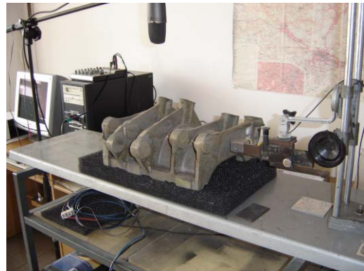
Fig.3. A general view of the test stand. Note a directional microphone for picking up of the acoustic field, a measuring rig with casting (magnesium alloy) placed in position, and a device for mechanical excitation of vibrations. The casting ready for testing is a 5-rib element made from magnesium AZ-7 alloy. The stand is also provided with a computer which records sounds from a mixer connected to the microphone.
