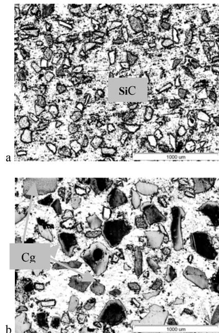
Fig. 3. Microstructure of AlSi12CuMgNi/SiC<sub>p</sub>+Cg heterophase ingot, OM: a) lower part of the composite ingot, b) upper part of the composite ingot.
