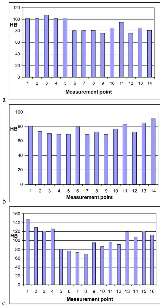
Fig. 7. Brinell' hardness on the cross section of composite ingots: a) AlSi12CuMgNi -Cg<sub>p</sub>, b) AlSi12CuMgNi -SiC<sub>p</sub>, c) AlSi12CuMgNi/SiC<sub>p</sub>+Cg<sub>p</sub>.
