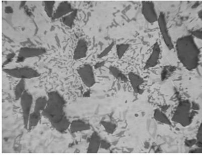
Fig. 4. Microstructure of AlSi12CuMgNi/SiC<sub>p</sub> composite ingot.
