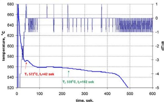
Fig. 5. Solidification curve of the AlSi12CuMgNi aluminium matrix alloy.
