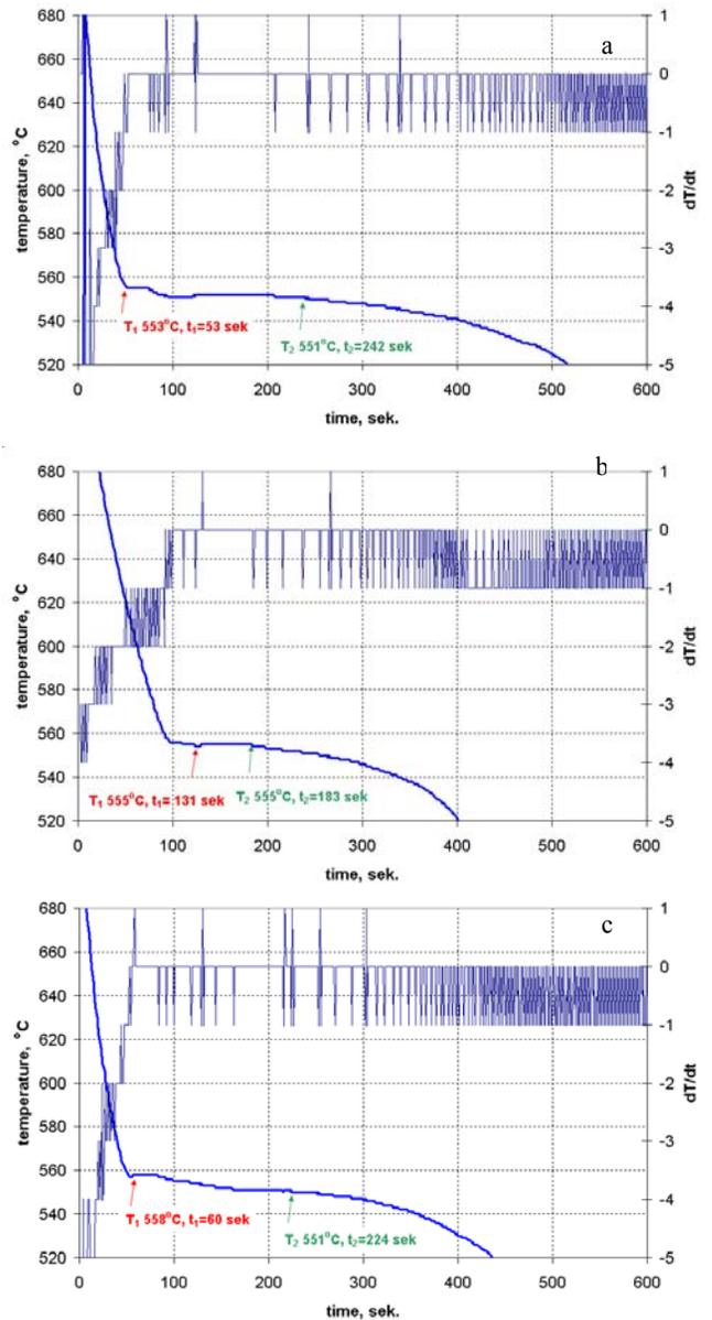
Fig. 6. Solidification curves of the: a) composite with glassy carbon (Cg) particles, b) composite with silicon carbide ceramic particles (SiC), b) AlSi12CuMgNi/SiC<sub>p</sub>+Cg heterophase composite.
