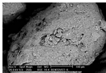
Fig. 2c. Model sand (sixth circulation) surface detail, SEM
