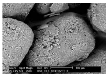
Fig. 2b. Model sand (third circulation) surface detail, SEM
