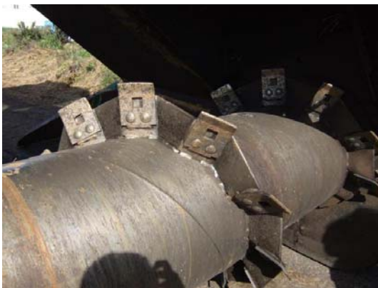
Fig. 2. Paddles on a rotor of the turning machine
