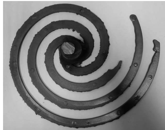
Fig. 2. Photographs of Archimedes spirals with wall thickness of 1, 2 and 3mm
