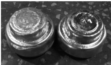
Fig. 1. Taking a sample to evaluate the porosity content and measuring the molten metal temperature with an immersion thermocouple –a). Samples for testing the alloy porosity content –b)
