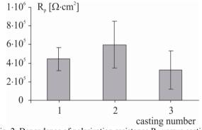
Fig. 2. Dependence of polarization resistance  $R_p$  versus casting number
