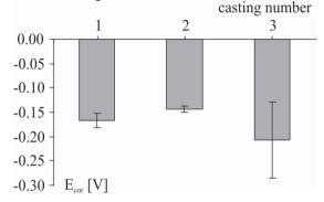
Fig. 1. Dependence of corrosion potential  $E_{cor}$  versus casting number
