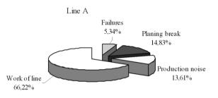
Fig. 5. Groups of causes of casting line stoppages within a year
