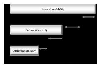
Fig. 4. Overall Equipment Effectiveness - O.E.E. (B/A: equipment availability, C/B: performance efficiency, D/C: quality rate)
