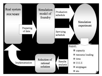
Fig. 2. Simulation of production systems
