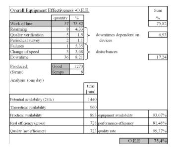
Fig. 7. Results analysis on the basis of simulation report
