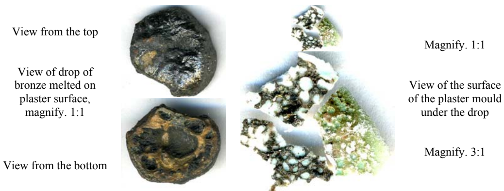
Fig. 8. View of the drop of the solidification bronze on plaster mould and the fragments of plaster mould from the side of the contact with the melted drop
