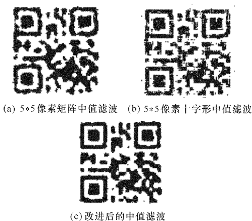
图3 116 * 116 像素图像的几种中值滤波效果比较图 Fig. 3 Comparison image of 116 * 116 pixel image with several median filtering effects
