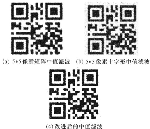
图4 377 * 377 像素图像的几种中值滤波效果比较图 Fig. 4 Comparison image of 377 * 377 pixel image with several median filtering effects
