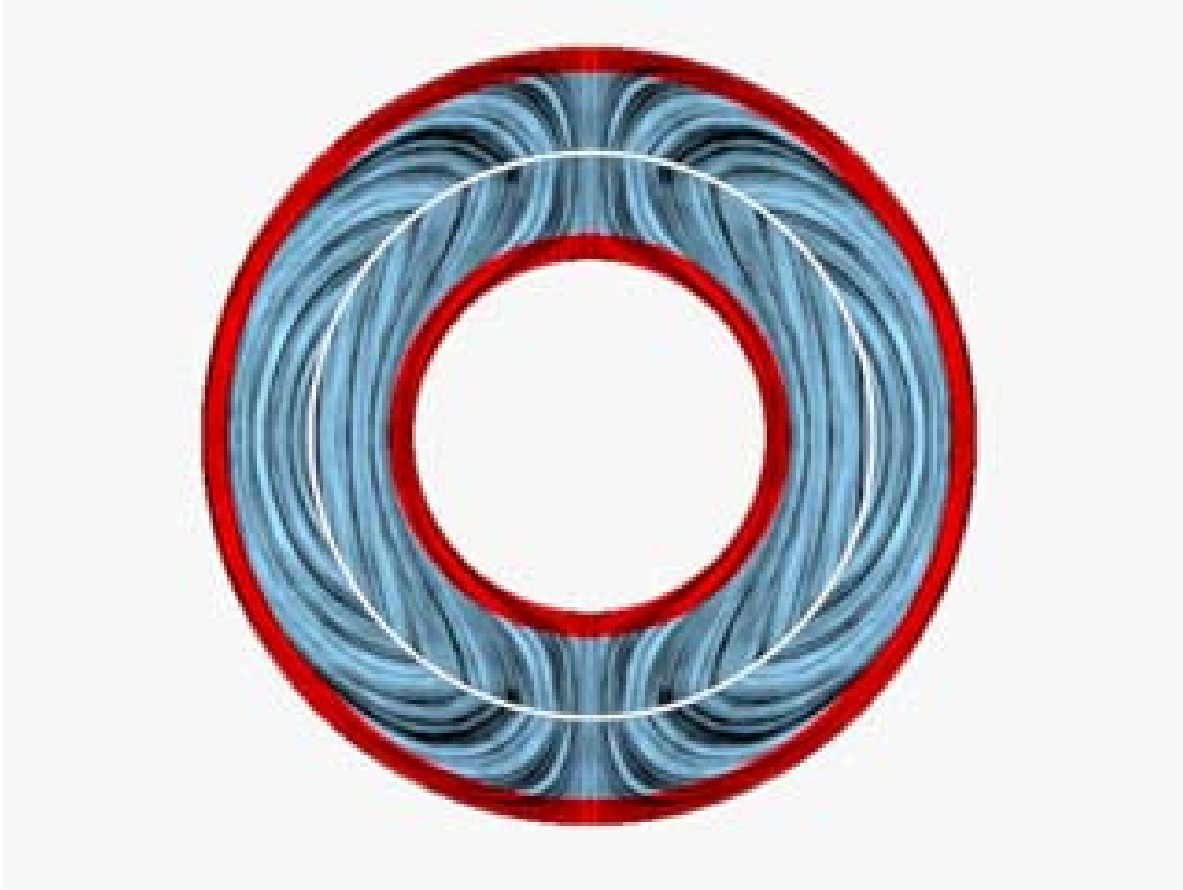
Figure 3: A line integral convolution representation of the magnetic field topology for a ramp turn-on in a time T = 0.1 a/c . We show the field at a time t = 0.5 a/c after the turn-on starting at t = 0 . The sphere is indicated by the silver circle.
