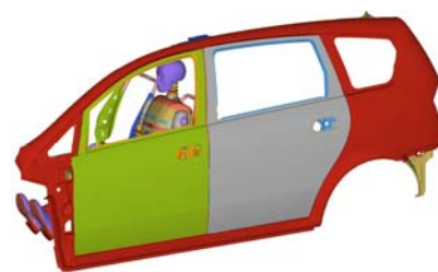
Fig. 5. Model of occupant injury criteria calculation
