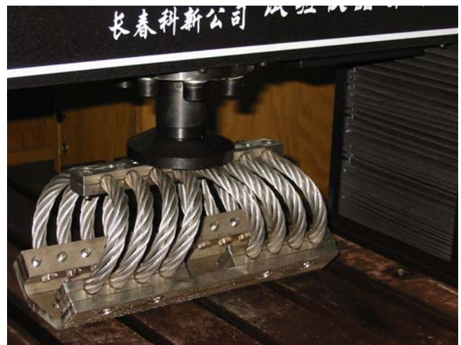
Fig.4 Steel rope spring in calibrating test
