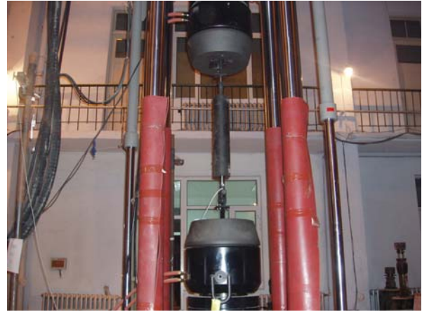
Fig.2 MR damper in calibrating test
