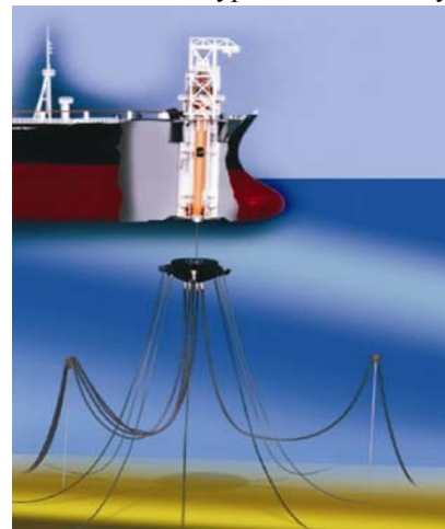
Fig.4 Buoy turret mooring (BTM) for internal turret
