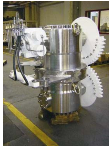
Fig.6 Hydraulically operated riser QC/DC valves
