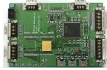
Figure 2: UFFO Data Acquisition (UDAQ) board
