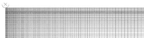
Fig. 2 Finite element model of a sandwich beam indented by a cylindrical indenter
