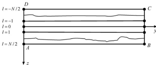
Fig. 2 The semi-continuum model for an ultra-thin beam
