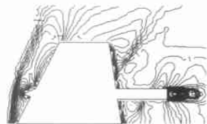
图 9 计算所得等 Ma 数线图 ( Ma = 1.2, x_0 = 18 ) Fig. 9 Mach contours of the fin with a bulge ( Ma = 1.2, x_0 = 18 )
