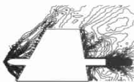
图 8 计算所得等 Ma 数线图 ( Ma = 1.5, x_0 = -38 ) Fig. 8 Mach contours of the fin with a bulge ( Ma = 1.5, x_0 = -38 )
