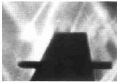
图 5 有鼓包舵的风洞实验照片 ( Ma = 1.2 ) Fig. 5 Picture of the fin with a bulge in wind tunnel ( Ma = 1.2 )
