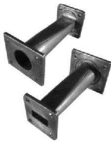
FIG. 1: Adaptors from rectangular (frequency X-band 8.2 GHz - 12.4 GHz; wavelength 36.6 mm - 24.2 mm) to circular waveguide and vice versa. The rectangular and circular guides have the same cut-off frequency of 6.5 GHz and the same dispersion relation. The inside guide dimensions are 10.16 mm · 22.86 mm and 27 mm diameter, respectively. The total adaptor length is 105 mm.
