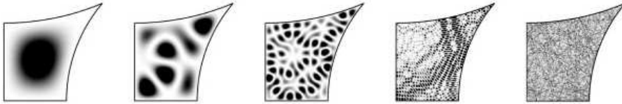
FIG. 7.16. Illustration of spatial distribution of the Dirichlet eigenfunction |u_m|^2 (shown as density plots: larger values are darker) with m = 1, 10, 100, 1000 and m \approx 50000 [38] (by A. Barnett, with permission).
