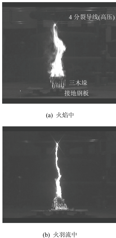
图2 四分裂导线在三木垛火焰中和火羽流中的击穿电弧 Fig. 2 Breakdown arc of four-bundle conductor in stable flame and fire plume of 3-crib fire
