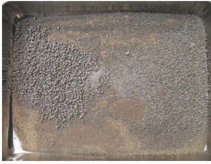
图4 实验后床料照片(50%石英砂+50%石煤灰; 900 °C) Fig. 4 Bed material after the experiment (50% quartz sand + 50% stone coal ash; 900 °C)
