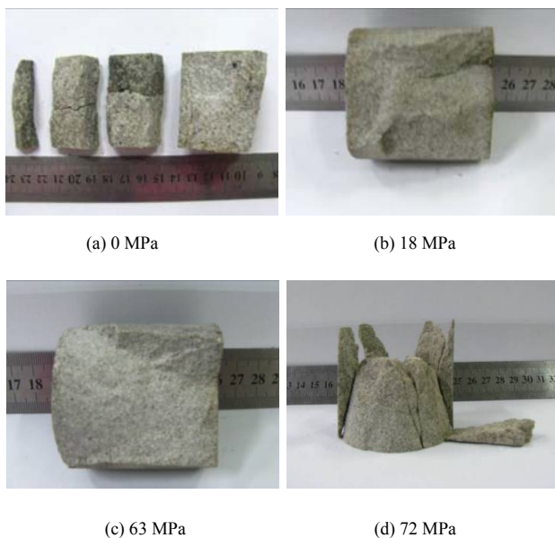
图 5 不同轴向静压下砂岩试样典型破坏形态 Fig.5 Typical failure forms of sandstone samples under different axial static pressures
