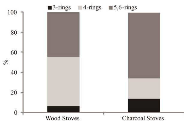
Figure 3. Ring number distribution of PM 2.5 bound PAHs in kitchens with wood and charcoal stoves expressed as percentage. 3-rings (PHE & ANT) represent lower molecular weight PAHs; 4-rings (FLT, PYR, BaA & CHY) represent medium molecular weight PAHs; and 5,6-rings (BbF, BkF, BaP, DBA & BgP) represents higher molecular weight PAHs.
