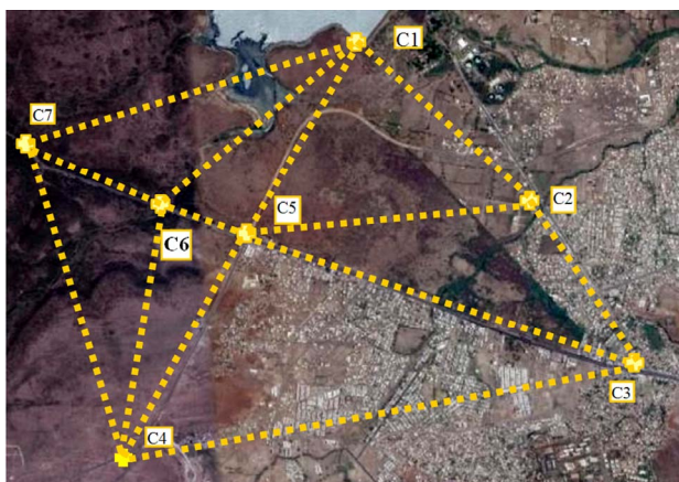
Figure 1. Area of Interest with Five triangles used for area computation study.
