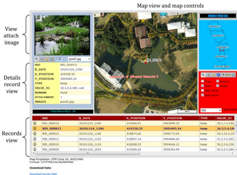
Figure 3. End user interface of Web-GIS for field survey data visualization in real-time.
