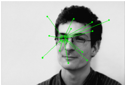
Fig.9. Testing for gaze movement for search the eye center from a group of initial gaze points in a random distribution.
