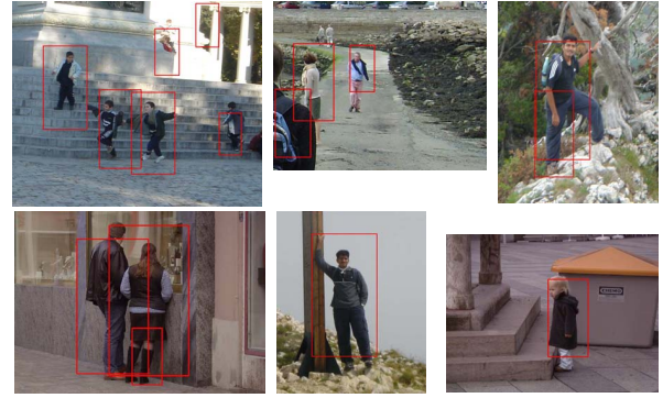
Fig. 7. Some detection results on INRIA dataset. Note that significantly overlapping detection windows are averaged into a single window.
