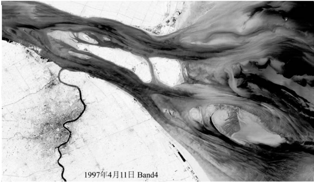
Fig. 6(a) Flow state of the sediment exchanges between the shoal and the channel in the north passage of Changjiang Estuary
