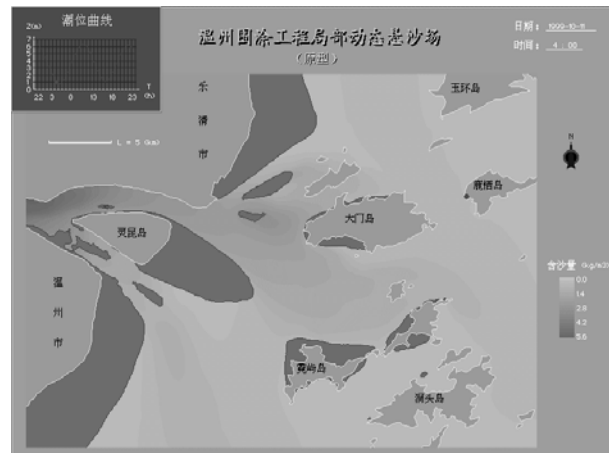
Fig. 6 Suspended sediment field at low slack water
