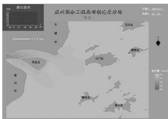
Fig. 7 Suspended sediment field transported by tidal flow at some time
