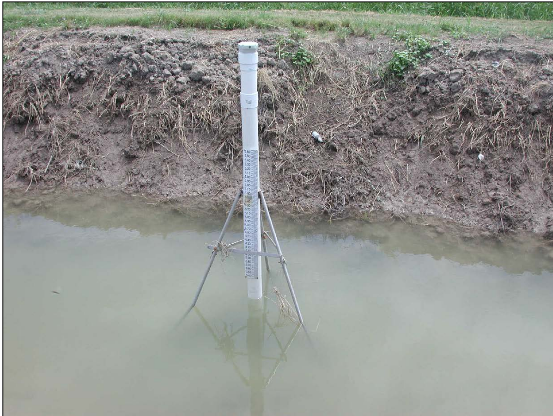
Figure 6. Staff gauge use to manual measure water levels.
