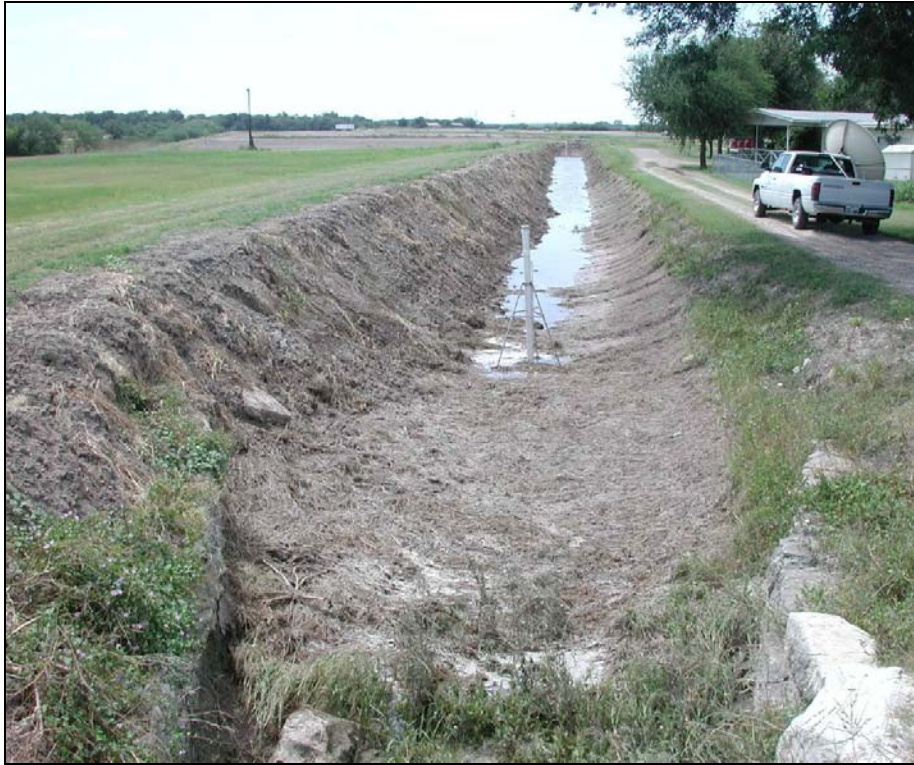
Figure 1. Test MA3, a segment of the unlined canal Lat. 8E.
