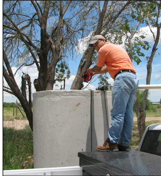
Figure 4. Askar is shown here measuring the drop in water level with the sounding meter.
