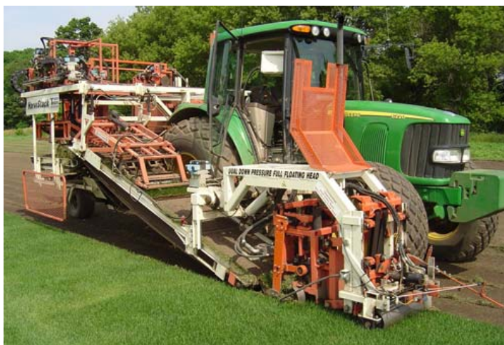
Figure 3. Sod harvesting equipment
