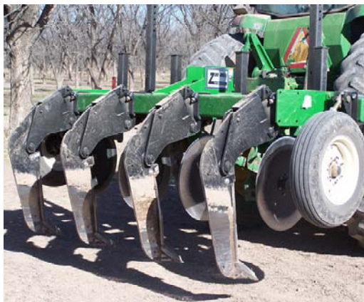
Fig. 5. Subsoiling shank penetrating 70 cm deep.
