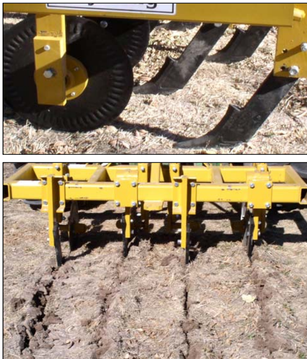
Fig. 4. A minimum-till surface chisel being tested for alleviating soil surface compaction in pecan orchards.
