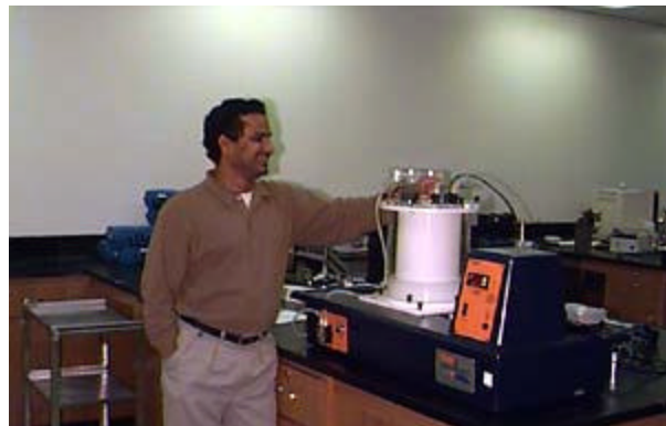
The literature search will be carried out by Raghava Kommalapati, shown here in his lab working with a unit that can simulate aeration for wastewater treatment.
