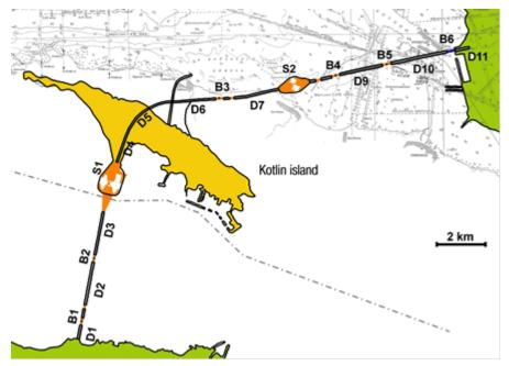
Figure 2: Layout of Dams (D1-D11), Sluices (B1-B6) and Navigation Openings (S1 & S2)
