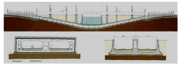
Figure 10: S1 Navigation Opening - tunnel sections
