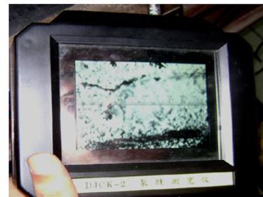
(c) DJCK-2 型裂纹测宽仪
