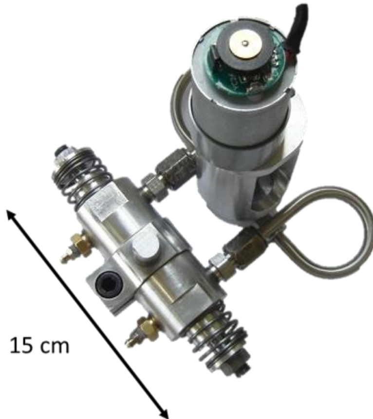
Figure 21. First generation fabricated damper and servo-valve used for control development.
