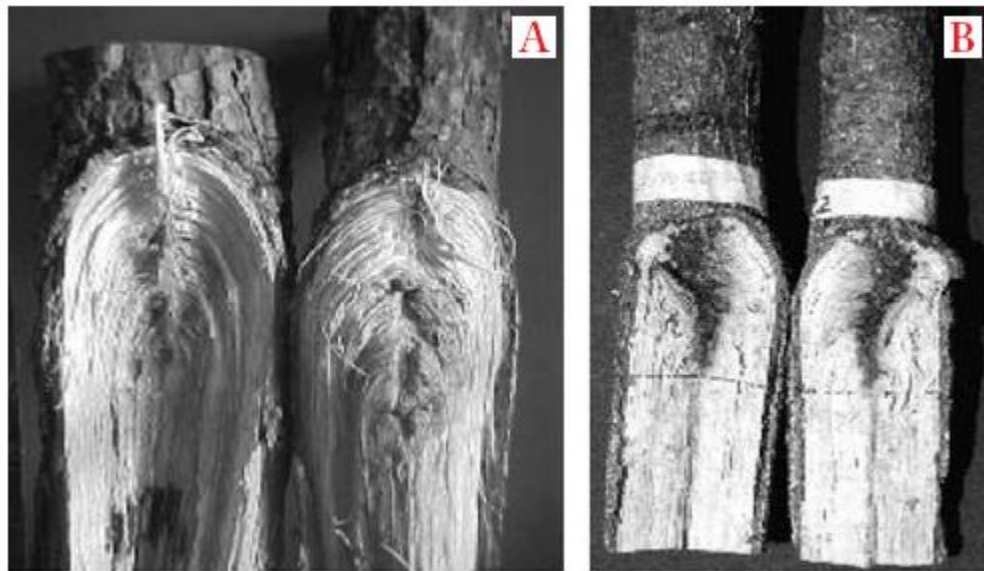
Figure 2.24: Examples of the failure modes for (A) the embedded branch failure mode, and (B) the flat surface failure mode (Kane et al. 2008).
