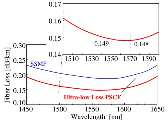
Fig. 4 Loss Spectra of PSCF and SSMF.
