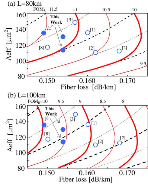
Fig. 2 Iso- $FOM_R$  as Functions of Loss and  $A_{eff}$  at Span Length of (a) 80km and (b) 110km.
