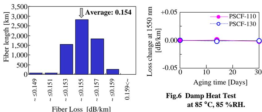
**Fig.5 Fiber Loss Distribution over 7,000km PSCFs.**
