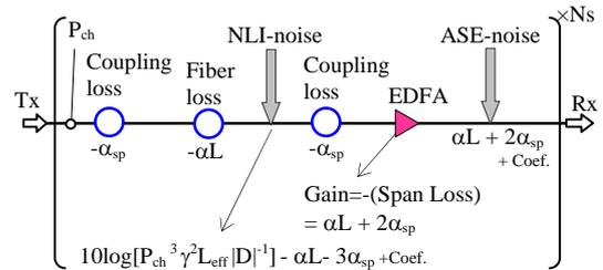
Fig. 1 Block Diagram of Considered Link.
