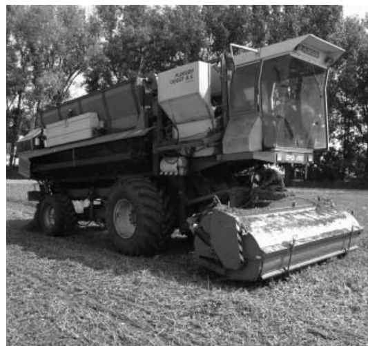
Fig. 1. (A) – Technological description of the release system: (1) main separator drum, (2) main release drum, (3) auxiliary release cylinders, (4) round side strips, (5) carry grain conveyor, (B) – view of the machine within work activities
