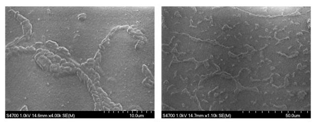
Figure 2. The SEM micrograph of Asaia bogorensis biofilm
