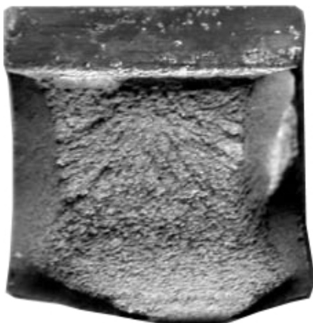
Figure 16. Fracture surface appearance of the steel 21MnTiB tempered at 200°C after the heat exposition of 100°C for 5000 h; test temperature -40°C
