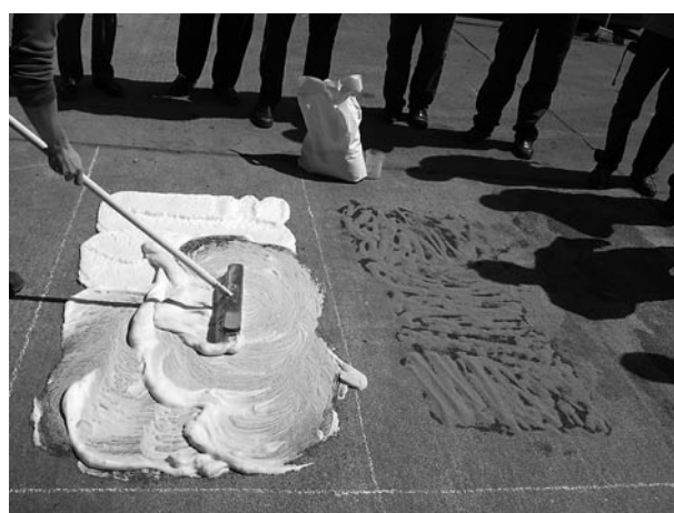
Figure 2. Decontamination process – comparing the decontamination with sorbent as opposed to reagent foam
