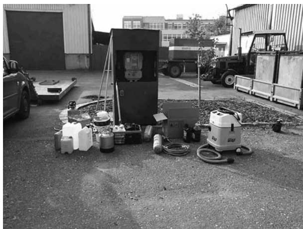
Figure 5. Equipment used for decontamination (from the left) – ordinary cleaning equipment, foam generator PZ 9, pressure bottle with compressed air, wet suction cleaner WAP
