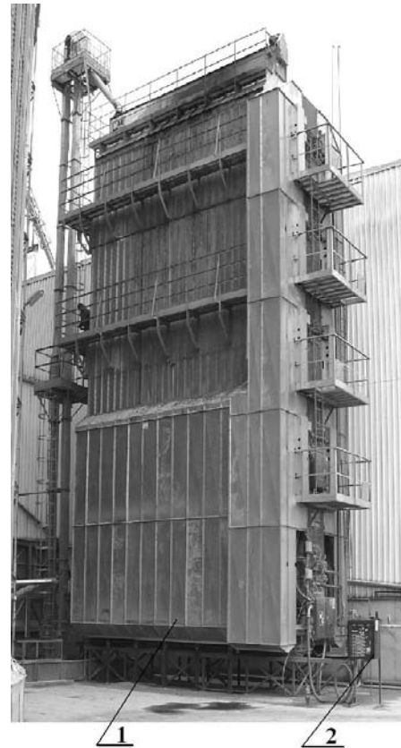
Figure 2. View of the examined MC 3180 dryer 1 – metal plating for recirculation, 2 – controlling console
